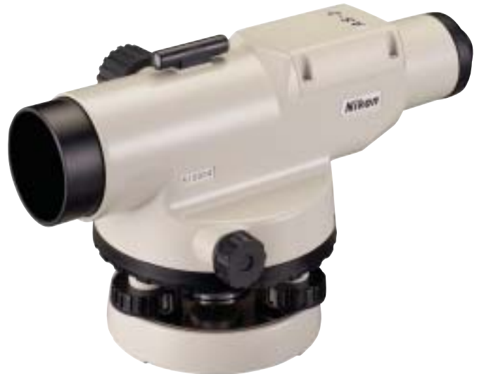
The waterproof telescope for the AS-2/AE-7 Series automatic levels is also airtight and filled with dry nitrogen gas to eliminate fogging in wet or humid environments.
