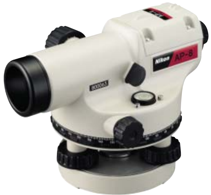
The lightweight, water-resistant AP-8, AC-2S and AX-2S automatic levels feature a built-in magnetic-dampened automatic compensator to level the line of sight.
