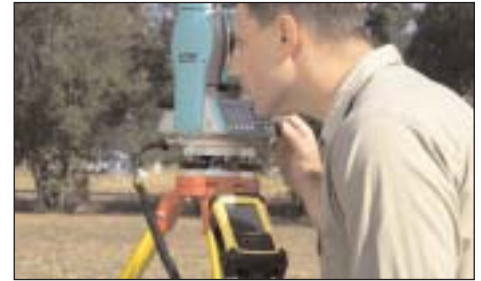
Connect a TDS Recon for more data collection capabilities You can expand your data collection capabilities by connecting a TDS Recon (shown) or Ranger data collector to the 502 Series total station.
